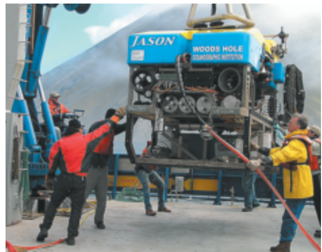
Figure 4. The remotely operated vehicle, Jason II was used to examine coral habitat at depths between 367 and 3000 meters.
