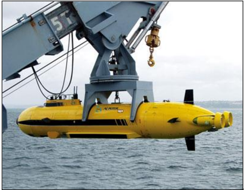
Figure 5: Autonomous underwater vehicles (AUV) are equipped with a suite of sensors and are programmed to operate independently of a support vessel for many hours. Some periodically come to the surface to download data.
